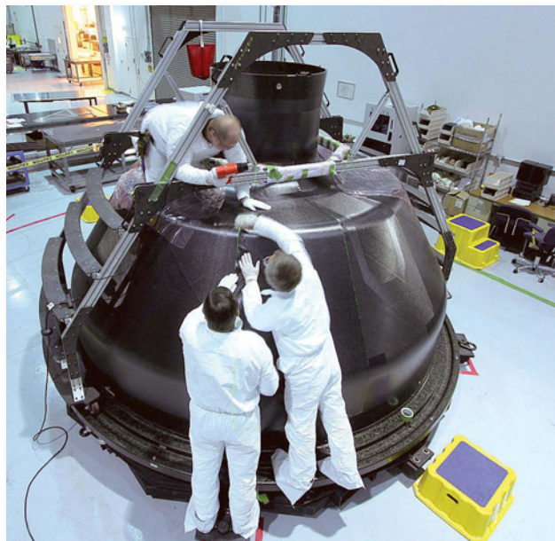
Fabricators at ATK in luka, MS, laying up plies of composite material to create the inner honeycomb sandwich skin of the NASA crew module. The plies are being laid up with the assistance of a laser projection system, which is driven by VISTAGY's FiberSIM software.
